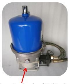
Mounting Bracket & Oil Drain to tank
