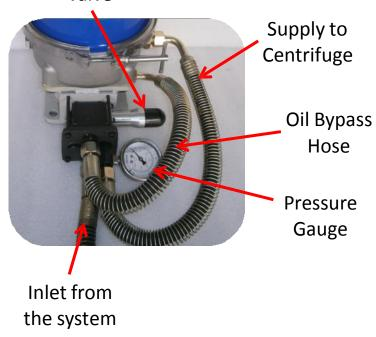
NOTE: To adjust the pressure, open black rubber cap & adjust pressure with Allen Screw. (Pressure not to raise beyond 7 Bar)
